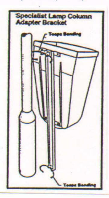
Fix onto lamp using Tespa banding through both top and bottom slots. Ensure banding does not cover inspection covers on lamp column.
